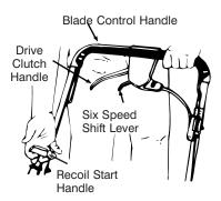
Figure 9-RECOIL START MODEL SHOWN
